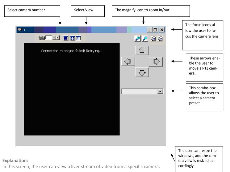
Select camera number: The user can select camera number by entering the camera number into a text box or pressing the left-right selector. Any change to the camera number will imminently cause the viewer to change to the request camera.
